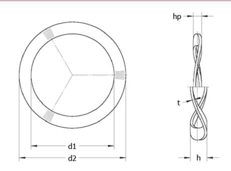
$\begin{array}{ll} d1 &= 60.70 \\ d2 &= 70.80 \\ F (N) at hp &= 260.0 \\ For bearing &= 6207, 6404 \\ h &= 3.4 \\ hp &= 1.45 \\ t &= 0.50 \\ Waves &= 5 \end{array}$
